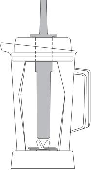
\*NOTE: Tampers have a small step on them. The step prevents contact of the tamper with the blades in the 48 oz. (1.4 liter) polycarbonate containers. Tampers cannot be used with one piece non-latching lid.
